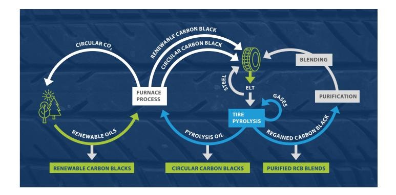
prime example is the fact that we use end-of-life tires as a raw material. We extract oil from the natural and synthetic rubbers from which the tires are made. And feasibility is improving constantly. The aim is to produce such a circular carbon black on a large scale from which new tires can be manufactured. This creates a cycle: a component of worn-out tires can be recycled back into new tires.
