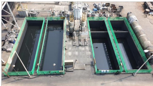
Recoverable water used in production process is collected in waste ponds such as the one shown here. They are reused mostly in the production process.
