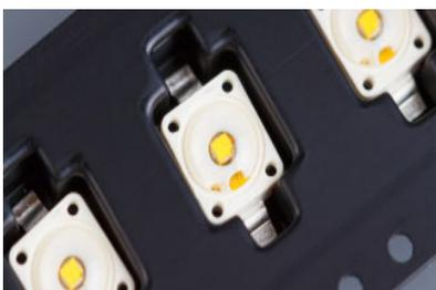
LEDs in conductive carrier tray
