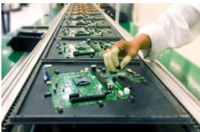
Transport boards for electronically sensitive devices
