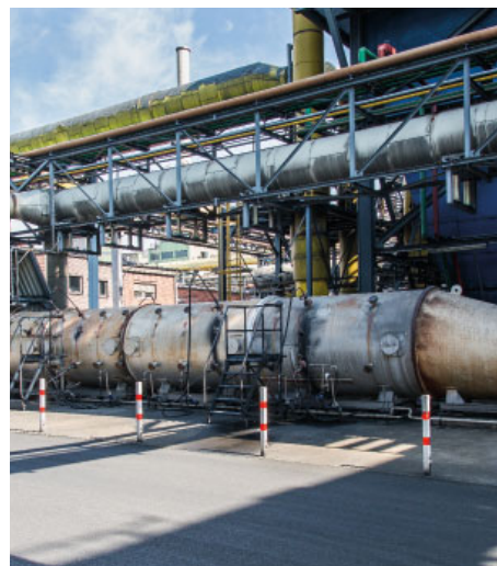
Figure 10: Furnace black reactor (section)
