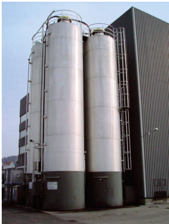
Storage silos for carbon blacks
