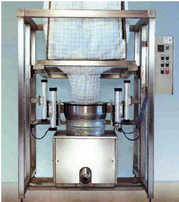
Mechanical agitation of an FIBC emptying device
