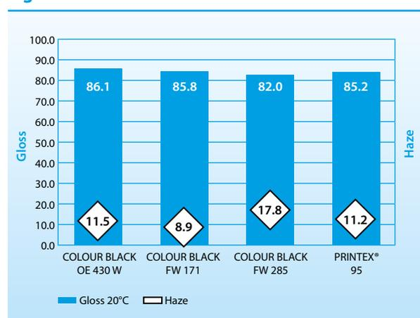
Results for gloss and haze of water-borne coatings based on COLOUR BLACK OE 430 W and several OEC high jetness specialty carbon blacks (stabilized with 70 % active to pigment). Letdowns were prepared using a coating system based on a commercially available 35 % PU dispersion (Alberdingk® U9800, Alberdingk & Boley GmbH). The final specialty carbon black concentration is 1.5 %.
