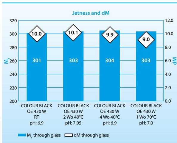
Colorimetric results of water-borne coatings based on COLOUR BLACK OE 430 W (directly and after storage of the COLOUR BLACK OE 430 W paste for two and four weeks at 40°C and 1 week at 70°C). Letdowns were prepared using a 1C PU coating system (Alberdingk® U9800). The final specialty carbon black concentration is 1.5 %.
