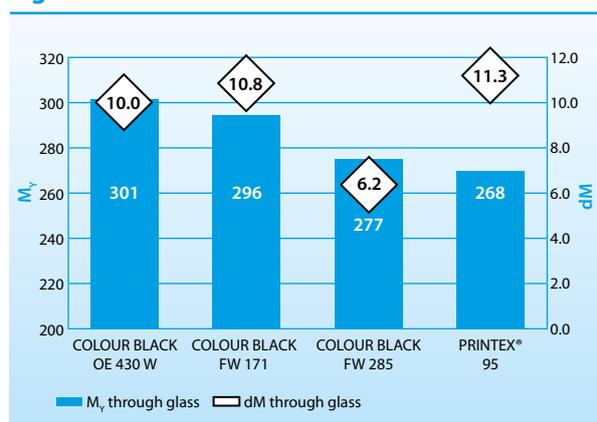
Colorimetric results of water-borne coatings based on COLOUR BLACK OE 430 W and OEC high jetness specialty carbon blacks (stabilized with 70 % active to pigment). Letdowns were prepared using a coating system based on a commercially available 35 % PU dispersion (Alberdingk® U9800, Alberdingk & Boley GmbH). The final specialty carbon black concentration is 1.5 %.
