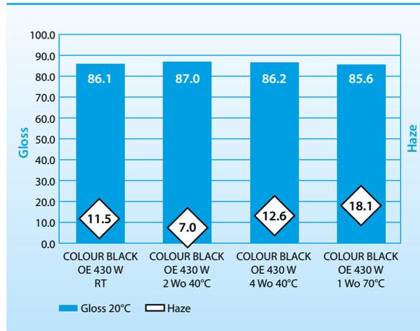
Results for gloss and haze of water-borne coatings based on COLOUR BLACK OE 430 W (directly and after storage of the COLOUR BLACK OE 430 W paste for two and four weeks at 40°C and 1 week at 70°C). Letdowns were prepared using a 1C PU coating system (Alberdingk® U9800). The final specialty carbon black concentration is 1.5 %.
