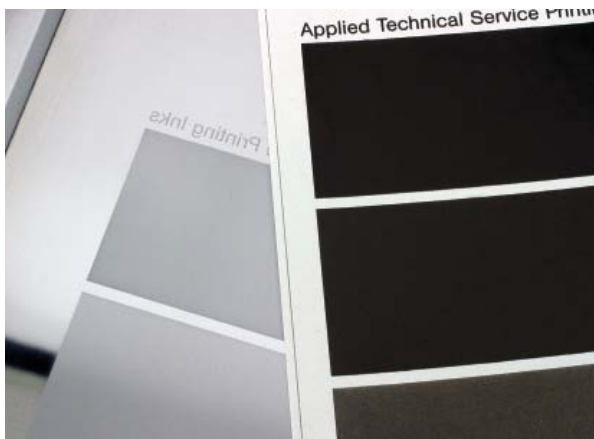
Single 3 Wedge Plate (60 lines/cm) and Print Results
