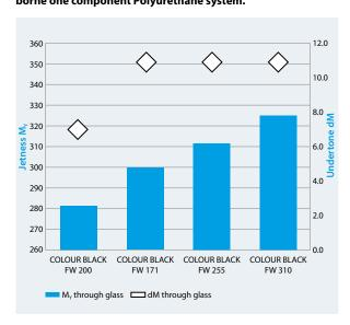
Figure 2 shows that in the tested water-borne coating system, COLOUR BLACK FW 310 achieves more than ten point higher jetness compared to the former best in class pigment COLOUR BLACK FW 255. The undertone is with more than ten as well on a very high level providing bluish undertone to the high jetness black coating.
