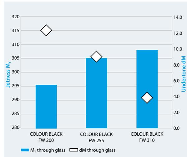
As demonstrated for water-borne coatings, as well in solvent-borne coatings the selection of the right additive and the right additive amount, is crucial. This is shown in figure 5. Deviations of more than 20 points of jetness can be found. Of course the findings will be completely different when using a different binder system. This is only to demonstrate that the formulation needs to be optimized with all ingredients.
