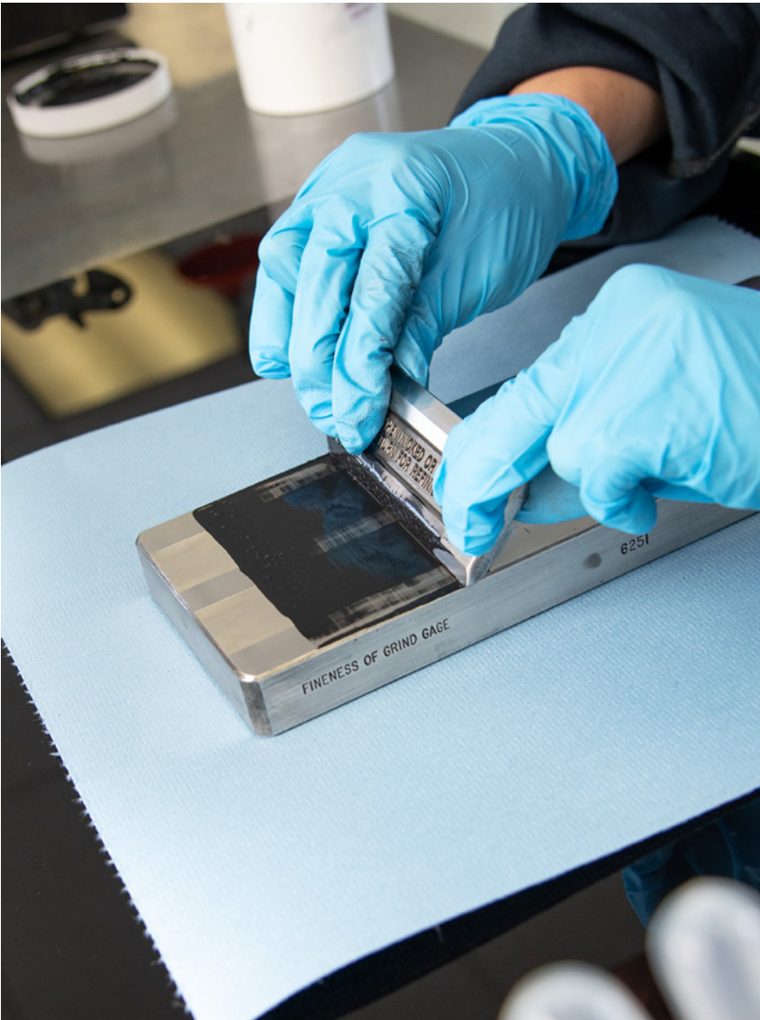
Testing carbon black in Orion’s lab in Carlstadt, New Jersey.
